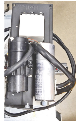
Tower Rear Relay & Capacitor
