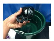
17 Rinse the nozzle components in lukewarm, clean water to remove soapy residue.
