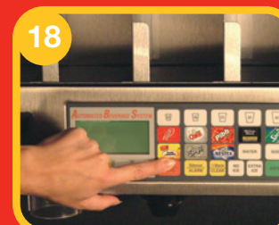
17 Wipe dirt and dust from the outside of the machine with McD APC solution and wipe dry with a soft, sanitized cloth. • Apply McD Stainless Steel Cleaner dressing to all exterior stainless steel surfaces and wipe dry with a paper towel. • Drink orders should be cleared before going back to "AUTOMATIC" mode. 18 Press the red "AUTO/MANUAL" button to place the ABS into "AUTO" mode.
