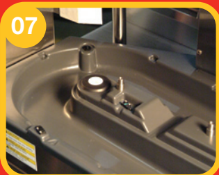
07 Make sure water deflector is properly installed; this will help prevent motor failures. (Order replacement if the deflector is missing.)
