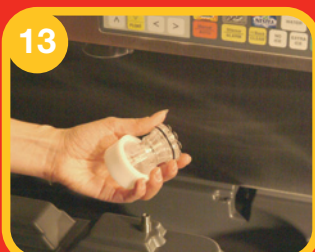
13 Remove collar from diffuser. • Check to see if syrup deflector is properly installed.
