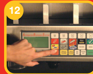
12 Clear drink orders by pressing the "UP ARROW" to highlight orders and pressing enter to clear orders. Refill ice chute. Return ABS unit to the "AUTO" mode by pressing the "AUTO/MANUAL" button.
