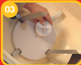
03 Remove the agitator retainer, disk, and the ice agitator assembly. Using McD APC and a long handled nylon bristle brush, clean the interior of the hopper, top cover, agitator and agitator cover. Rinse all with clean water. Prepare sanitize solution by adding one packet of McD Sanitizer to 2 1/2 gallons of lukewarm water in a clean sanitized bucket.
