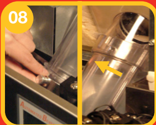
08 Pull the locking pin out and rotate the ice chute clockwise approximately 1 inch and pull down the ice chute.
