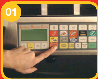
01 Press the red "AUTO/MANUAL" button to place the ABS unit into "MANUAL" mode.
