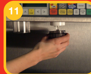
11 Prepare sanitize solution by adding one packet of McD Sanitizer to 2 1/2 gallons of lukewarm water in a clean sanitized bucket. • Remove the nozzle from the dispenser by turning and pulling down. 12 Remove the diffuser from the valve by pulling down. Place the nozzle and diffuser in the Sanitizer solution.
