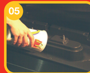
05 Pour warm (NOT HOT) water down drip tray drain. Flush the drip tray using carbonated water. Hot water or coffee will crack drip tray.
