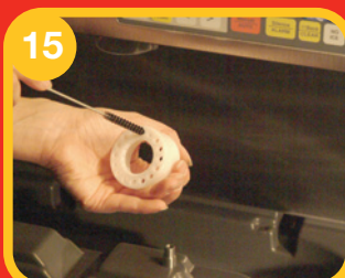
14 Clean the diffuser and nozzle using the nylon brush. Rinse with lukewarm water. • Reinstall the diffuser and nozzle. Ensure they are located correctly in the machine. • Dirty components can cause excess foaming.
