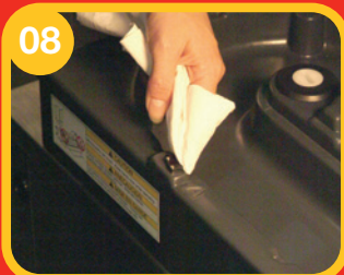
08 Roll the end of the paper napkin into a point and dip into the carbonated water and wipe both sensors. CAUTION: Never use a cleaning cloth, brush or abrasive cleansers on sensors.
