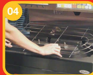
04 Remove the grille from the drip tray and clean with warm soapy water.
