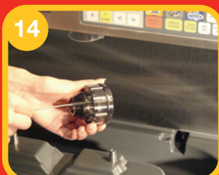
14 Clean the diffuser and nozzle using the nylon brush. Rinse with lukewarm water. • Reinstall the diffuser and nozzle. Ensure they are located correctly in the machine. • Dirty components can cause excess foaming.
