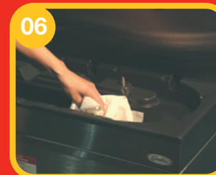
06 Wipe down the drip tray area, splash panel and clean any spills from the machine exterior using McD APC with a clean cloth.
