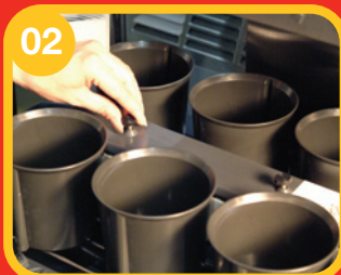
02 Loosen the screws (3) that retain the cup conveyor cover.
