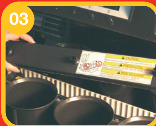
03 Remove the conveyor cover and conveyor assembly. Do not carry conveyor by cup holder.
