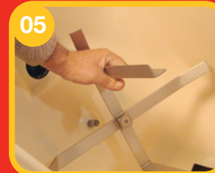
05 Using McD Sanitizer and a soft, sanitized cloth, wipe the interior of the hopper, top cover, agitator, and agitator cover. Reinstall the agitator retainer, disk, and the ice agitator assembly.
