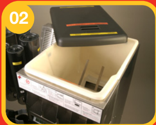
02 Remove the top cover and set it aside. Remove and discard all the ice from the hopper. If necessary, pour clean, potable water slowly into the hopper to assist in melting the ice.
