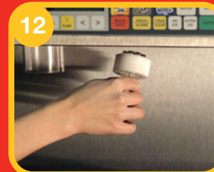
11 Prepare sanitize solution by adding one packet of McD Sanitizer to 2 1/2 gallons of lukewarm water in a clean sanitized bucket. • Remove the nozzle from the dispenser by turning and pulling down. 12 Remove the diffuser from the valve by pulling down. Place the nozzle and diffuser in the Sanitizer solution.
