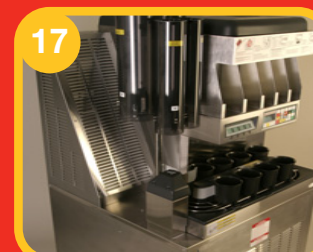
17 Wipe dirt and dust from the outside of the machine with McD APC solution and wipe dry with a soft, sanitized cloth. • Apply McD Stainless Steel Cleaner dressing to all exterior stainless steel surfaces and wipe dry with a paper towel. • Drink orders should be cleared before going back to "AUTOMATIC" mode. 18 Press the red "AUTO/MANUAL" button to place the ABS into "AUTO" mode.
