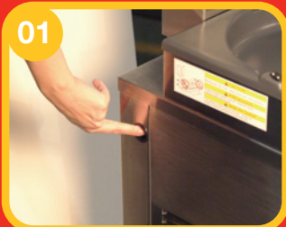
01 Turn ABS unit power switch "OFF". CAUTION: Unit will agitate if the ABS is left "ON".
