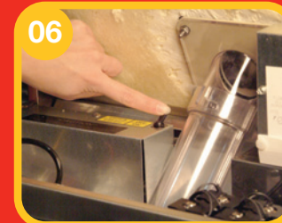
06 Turn manual ice gate switch "OFF" to relieve pressure on ice gate cylinder.
