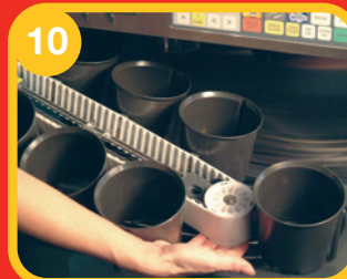
10 Clean the conveyor assembly using luke warm soapy water. • Do not use hot water or place in dishwasher. Rinse with plain water. • Reinstall the grille and conveyor assembly.
