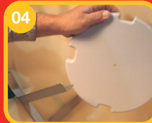
03 Remove the agitator retainer, disk, and the ice agitator assembly. Using McD APC and a long handled nylon bristle brush, clean the interior of the hopper, top cover, agitator and agitator cover. Rinse all with clean water. Prepare sanitize solution by adding one packet of McD Sanitizer to 2 1/2 gallons of lukewarm water in a clean sanitized bucket.
