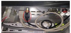
On the back of the display, unplug the black USB connection and plug in your USB flash drive containing your video file(s).
