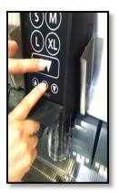
All LED lights will start blinking. After 5 seconds, the first light to the left (L1) will flash.
